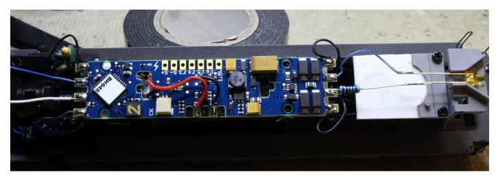
This is an example (without the insolation) of how to connect the headlights.
