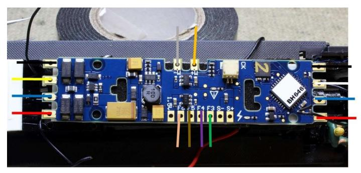
This shows the colour connections for the Tsunami 2.
